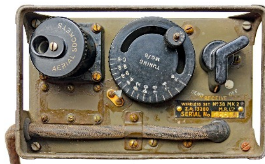
Front panel view of Wireless Set No. 38 Mk. 2 showing the large aerial socket opening where the Wired Wireless Adapter No. 1 was inserted.
